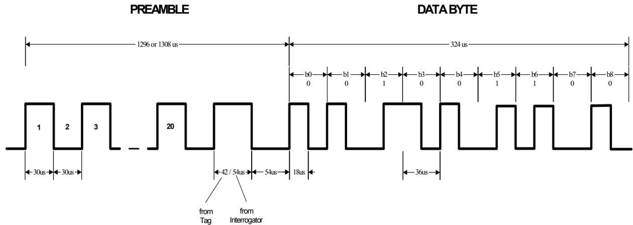
Pulse width in microseconds. Data byte transmitted significant bit first. Byte shown is code 0x64.
